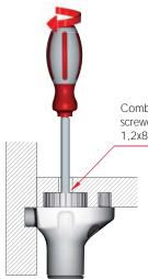
Combi slot for S6mm allen wrench or blade screwdriver 1x5,5 mm (LOWER CAVITY) or 1,2x8 mm (UPPER CAVITY).
